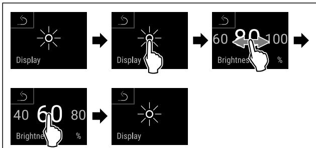
Fig. 133 Example illustration: Switch from 80 % to 60 %.
