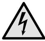
The symbol is located on the back of the appliance near the alarm relay and indicates the following danger: **Electric shock!** Even if an appliance is disconnected from the mains there may still be extraneous voltage. Do not remove sticker.
